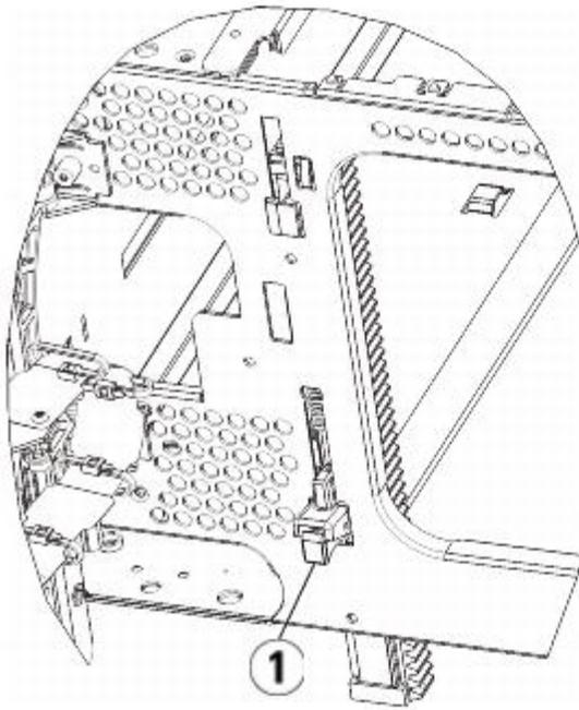
**1 Y-rail in unlocked, functional position**
