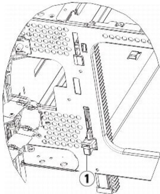
**1 Y-rail in unlocked, functional position**
