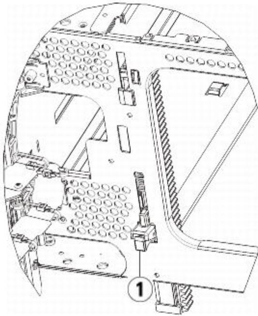
**1 Y-rail in unlocked, functional position**
