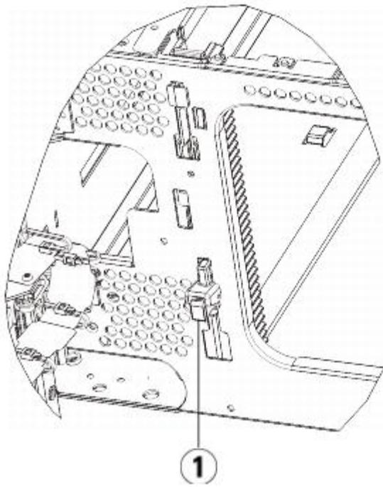
**1 Y-rail in locked, non-functional position**
