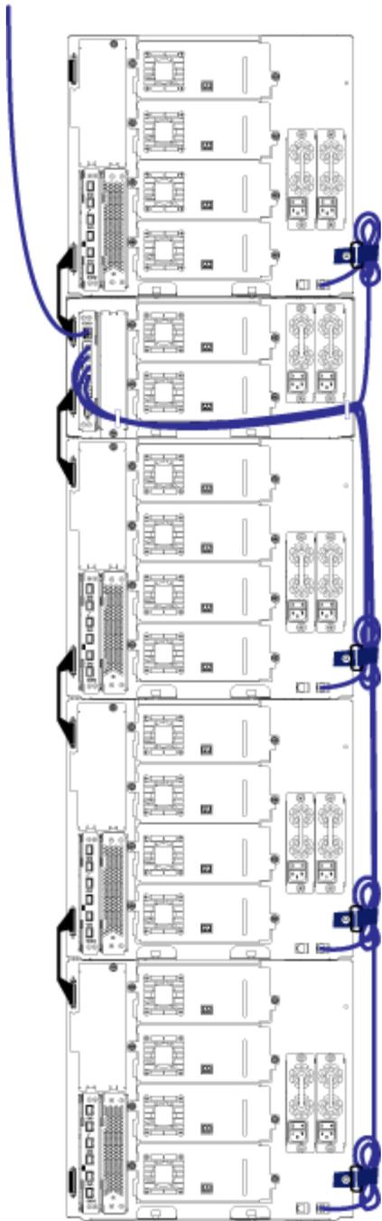
[Figure 14](#) shows how a 41U library would appear with power, Ethernet, and fibre cables installed and managed according to these guidelines.
