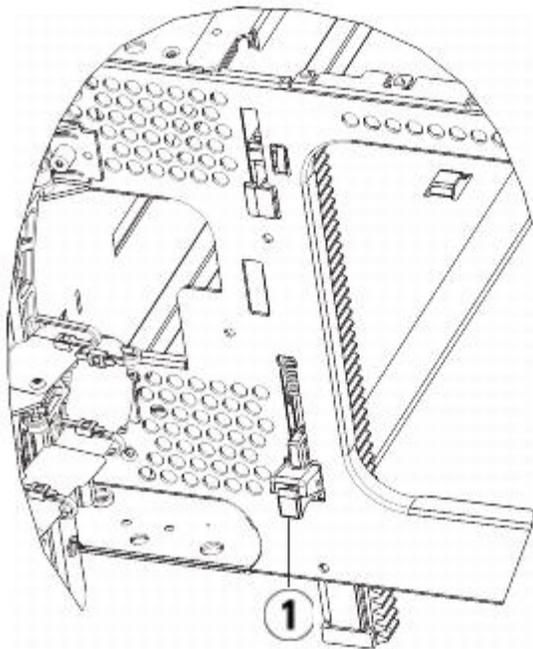
**1 Y-rail in unlocked, functional position**
